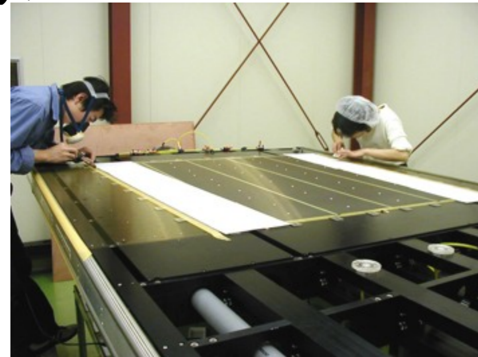
Manufactured at KEK: ~1000 wires being soldered
